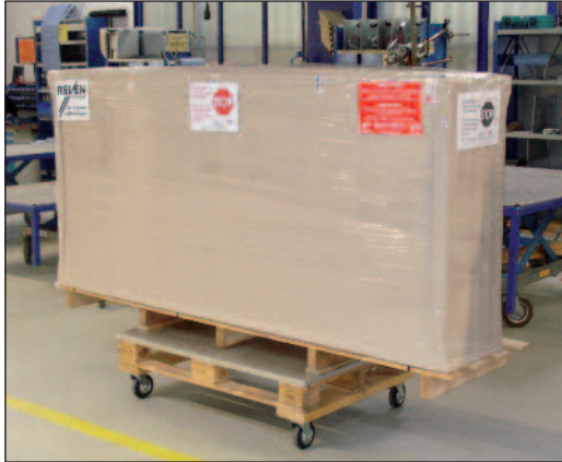
Fig.: transport position, supported on the longitudinal side
