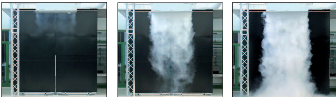
Visualization of the supply airflow behavior in the kitchen space when using a REVEN® ECOJET® unit, installation height = 3.50 m.
